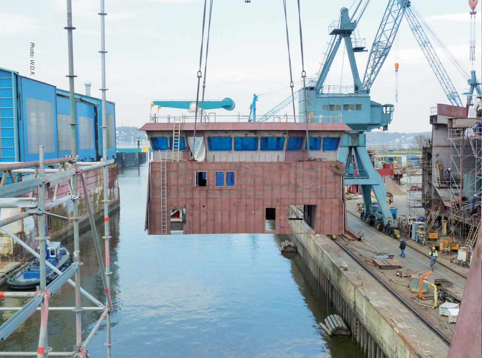
The implementation of sectional ship building was a cornerstone of Sietas' recent restructuring program. Here the prefabricated deckhouse and bridge of the M/V "Uthlande" are just being lifted onto the hull.
