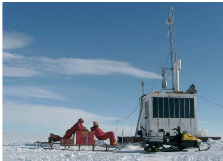
▲ WS-0,30A8 producing power for whale-noise recording device in Antarctica.
