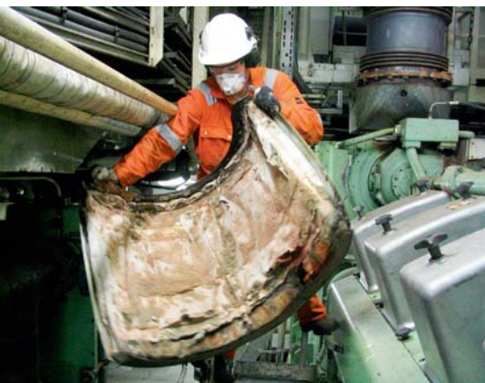
The pictures show how well Adi-XP® insulates exhaust pipes on a marine engine compared to a traditional insulation system, notice the damaged insulation.
