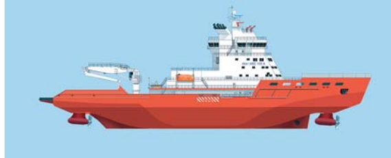
Aker ARC 100 design, the world's first oblique icebreaking emergency and rescue vessel BALTIKA can break sideways 50 m wide channel in 0.6 m thick ice.
