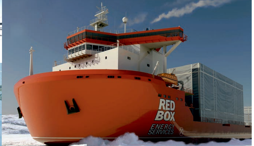
Aker ARC 100 design, the world's first oblique icebreaking emergency and rescue vessel BALTIKA can break sideways 50 m wide channel in 0.6 m thick ice.
